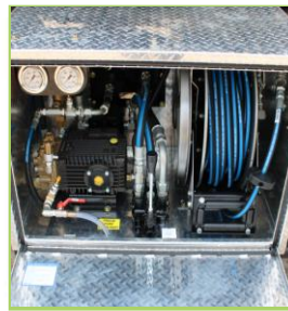
Hydro Excavation Package
