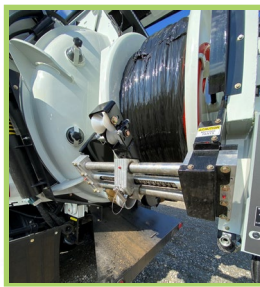
Tank Door, Hose Reel & Hose
