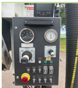
Rear Operator Controls
