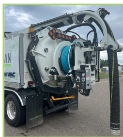
Tank Door, Hose Reel & Hose
