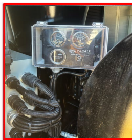
Air Excavation Controls
