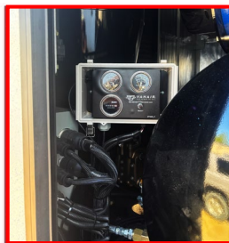
Air Excavation Controls
